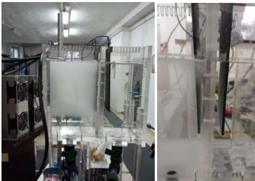
Figure 1. Laboratory electrochemical reactor with graphite electrodes for water pH control
