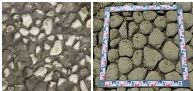
Figure 4. Samples of the river bed material – left fish pass on the Hron River, right on the Turiec River
