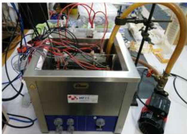
Figure 1. Modified ultrasonic bath used as an EC reactor in this study
