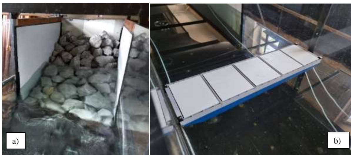
Figure 1. Photographs of a) the dissipation chamber at the end of the wave flume and b) the model of the BRK 5320 floating breakwater model with 4 mooring ropes
