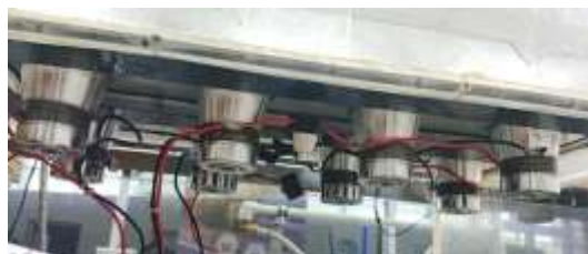
Figure 4. Ultrasonic transducers attached on the underside of the reactor [47]
