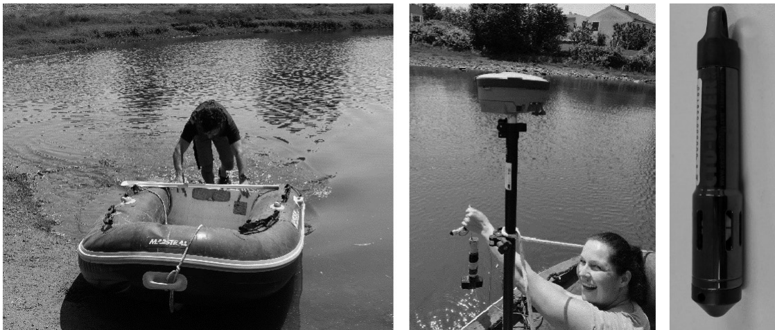
Figure 5. Equipment used for the bathymetry measurement (from left to right): Inflatable boat, Topcon positioning system HiPer V and CTD – diver [7]
