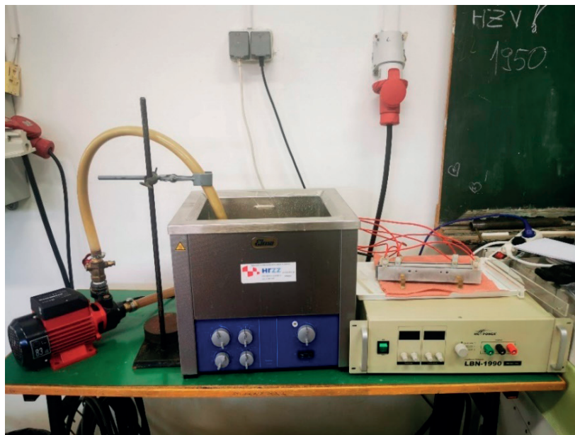
Figure 2. Modified ultrasonic bath with recirculation, laboratory power supply and aluminium electrodes
