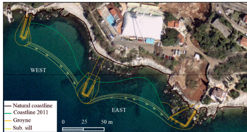
Figure 2. Historical coastline from aerial images from 1968 (black), the coastline of the artificial beach constructed in 2011 (green), constructed submerged sill (yellow) and groynes (orange)
