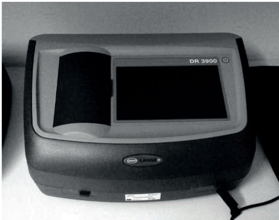
Figure 6. Equipment used for water quality measurement: Spectrophotometer – HACH DR 3900 [7]
