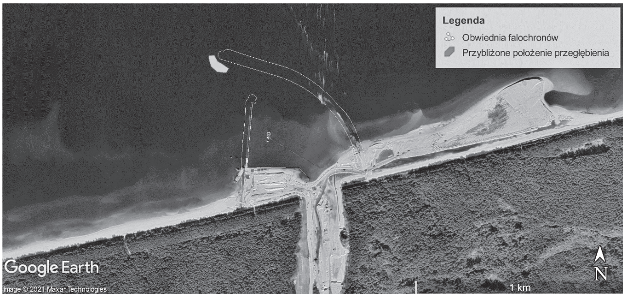
Figure 1. Approximate location of the scour (gray stain) near the head of the eastern breakwater (bright lines). Satellite image from September 2020
