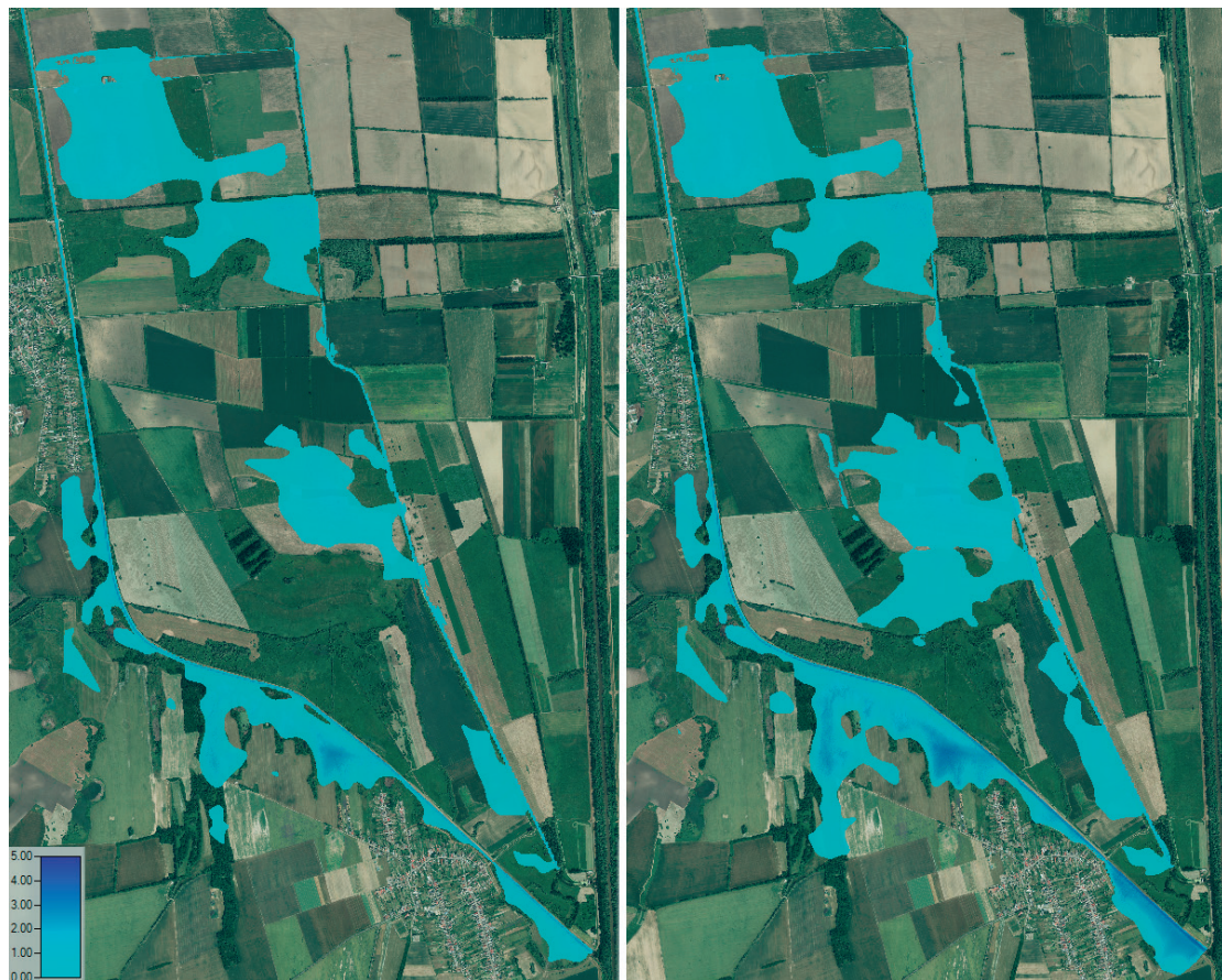
Figure 6. Flooded area at Q_{20} flood wave, left side – open flood gate, right side – closed flood gate
