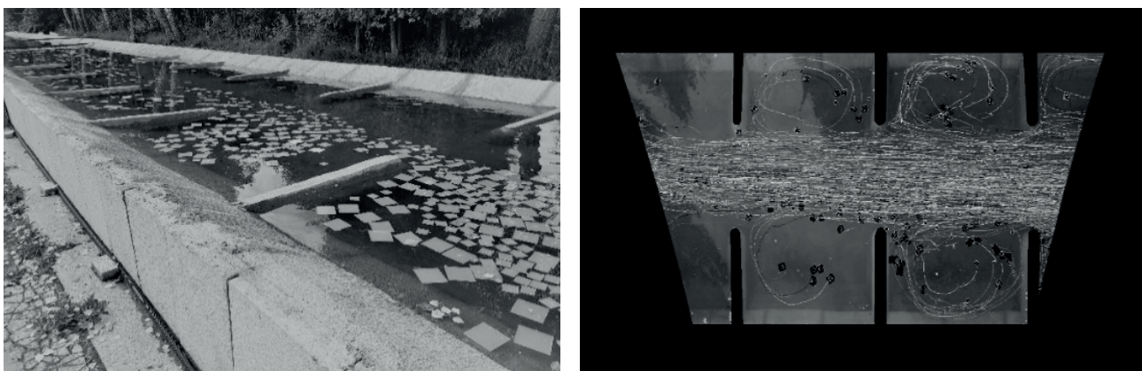
Figure 1. Exemplary photo from experiments with plastic tracer (left) and results from the PTV analysis (right)
