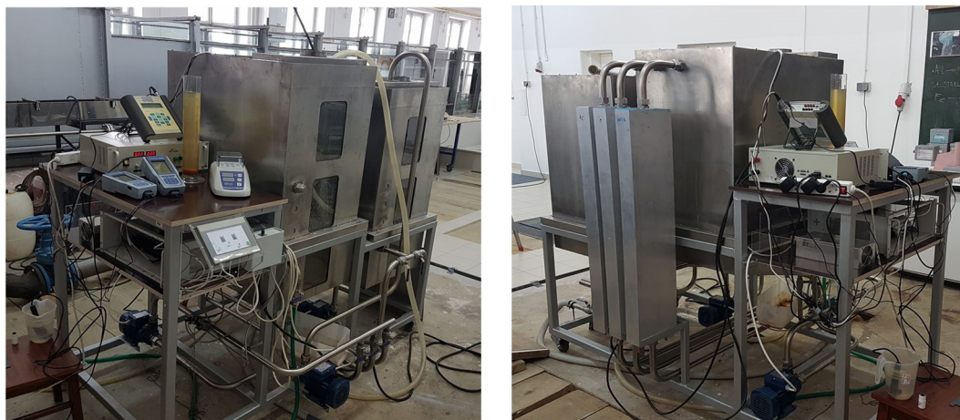
Figure 2. Electrocoagulation pilot device installed at the Faculty of Civil Engineering (University of Zagreb) (left - front of the device, right - back of the device)
