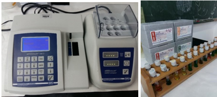
Figure 4. Photometric device NANOCOLOR 500D with samples after measurement
