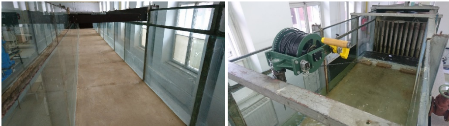
Figure 2. Hydraulic flume (left), hinged flap gate (right).
