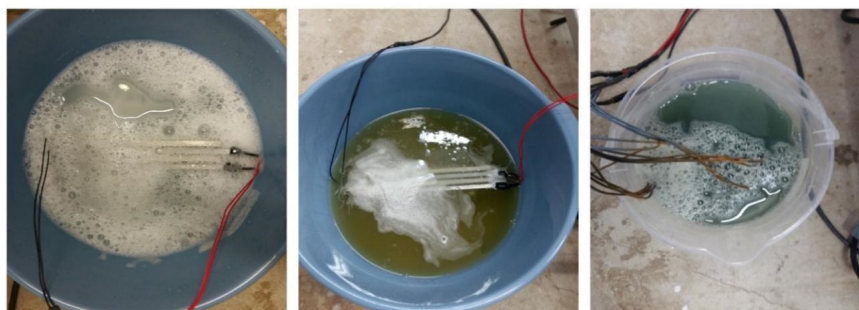
Figure 2. Electrodes in operation in 5-liter volumes in plastic containers
