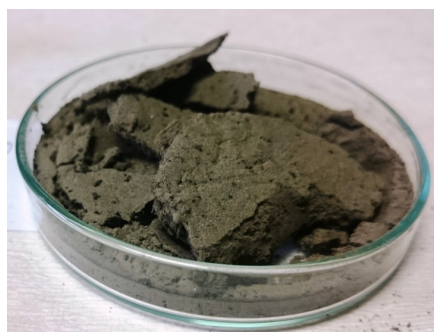
Figure 2. Example by formed and frangible biopolymer crust in Petri dish
