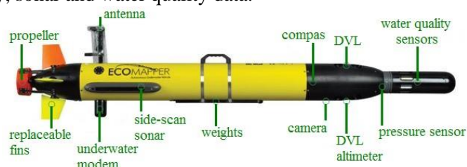
Figure 1. YSI EcoMapper side view (YSI, 2009)
