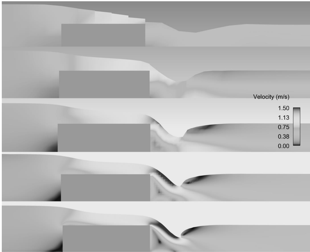
Figure 5. Accuracy of CFD for different mesh resolution varying from 0.1m up to 0.00625m
