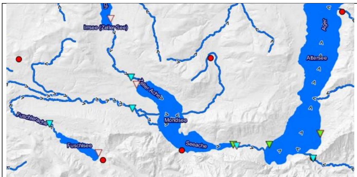
Figure 1. The hydrological system of lake Mondsee including hydro-meteorological gauges (red .. rain gauge, blue ... discharge, green ... stage, white ... water temperature).
