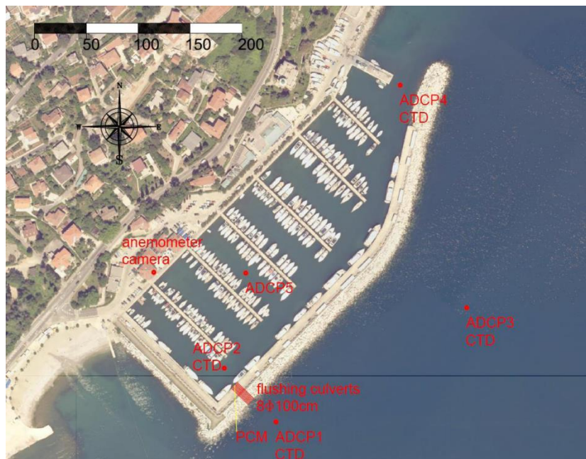
Figure 1. Layout of measuring devices in small harbour Opatija; ADCP- sea current profiler, CTD-salinity; PCM-discharge in flushing culvert
