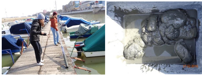
Figure 2. Sampling extraction using sediment core sampler type Beeker and sediment samples
