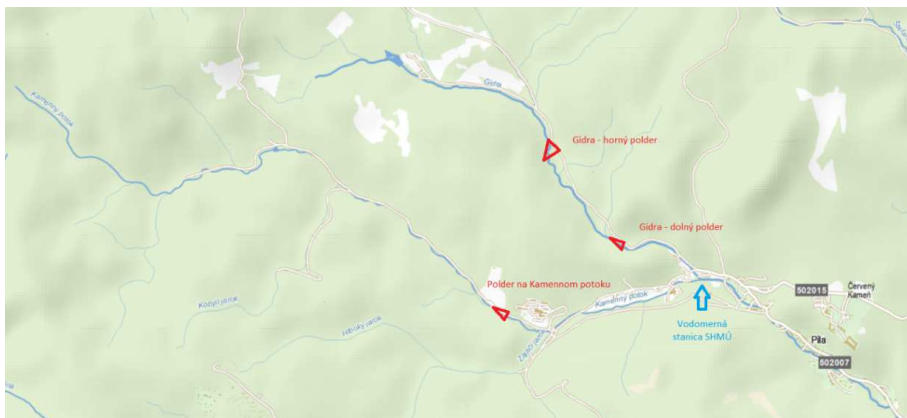
Fig. 6 Map of streams and their inflows and proposed detention reservoirs over the Píla town
