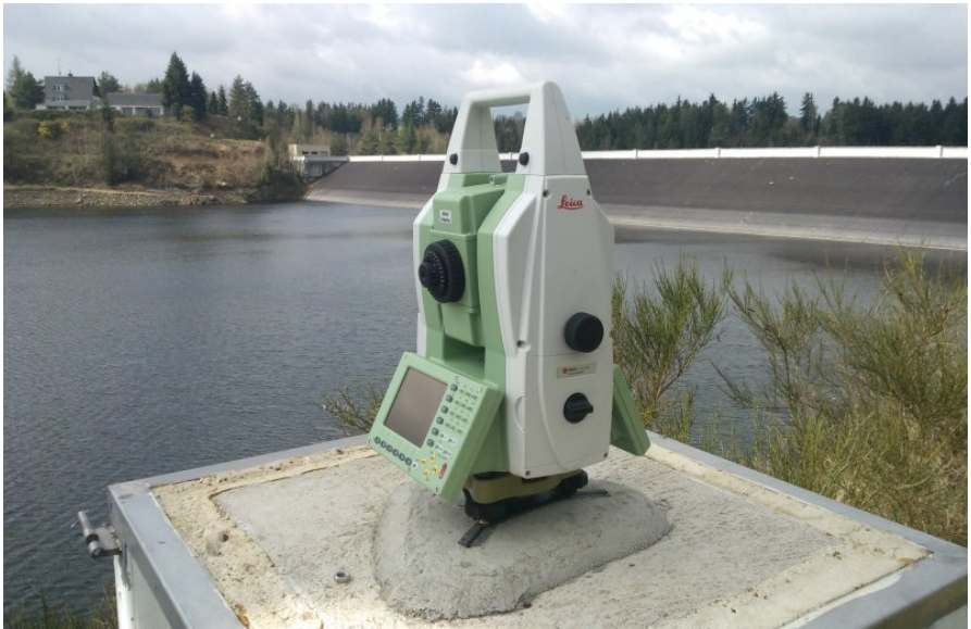
Fig. 1 Leica TM30, Stanovice dam
