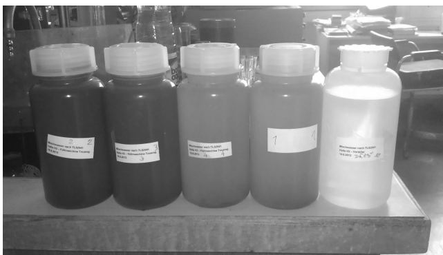
Fig. 1 Visual comparison of the rainwater (right) and the runoff from the green roof model (model with sludge incorporation – two samples most left, without the sludge – two samples in the middle)
