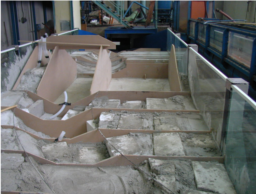
Fig. 1 The modelling of the river bed and dam
