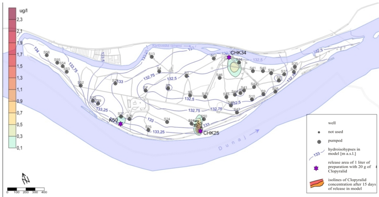
Fig. 3.5 Isolines of Clopyralid concentration in groundwater 15 days later since single point release [ \text{ug.l}^{-1} ]
