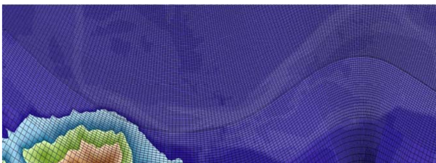
Fig. 13 Orthogonal curvilinear grid of the model with bathymetry
