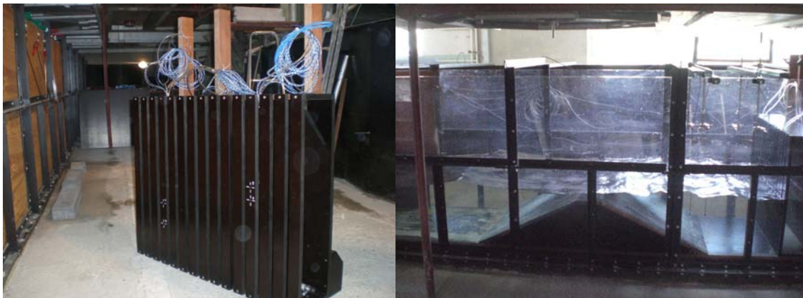
Fig. 7. Photographs of submerged low crested structure (LCS) positioned in channel for crown submergence F=0.055\text{m}
