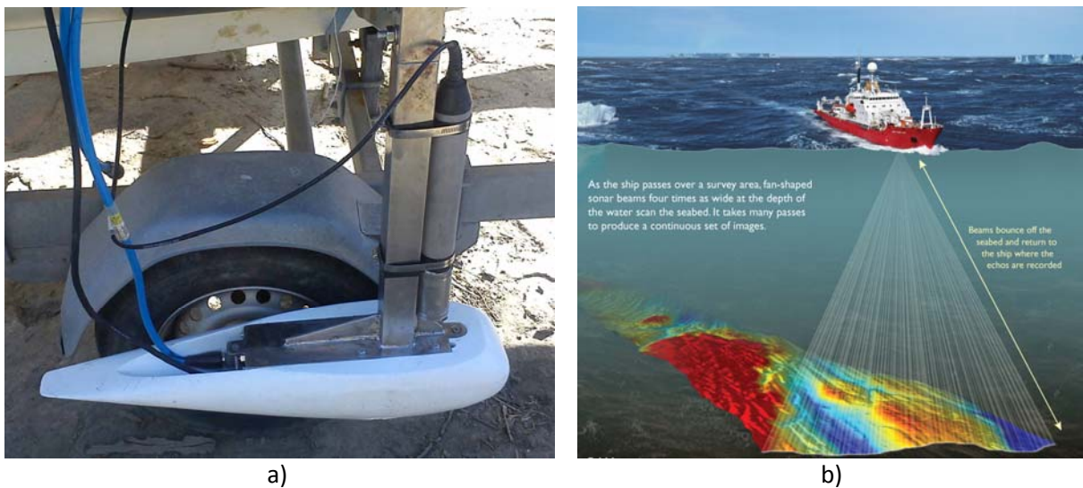
Fig. 3 Multibeam echo sounder: a) boat mount, b) operation scheme.
