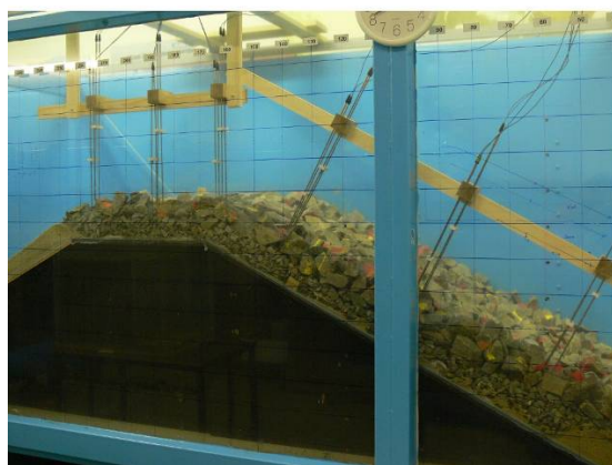
Fig.3 Hydraulic model of the dike [6]
