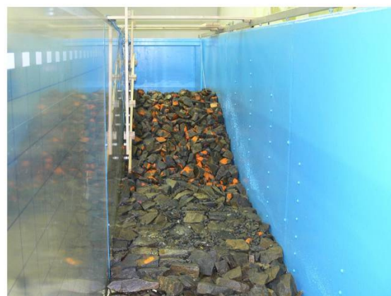
Fig.3 Hydraulic model of the dike [6]
