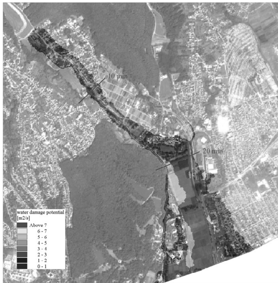
Fig. 7. Flooded area, water damage potential and travel times of wave front
