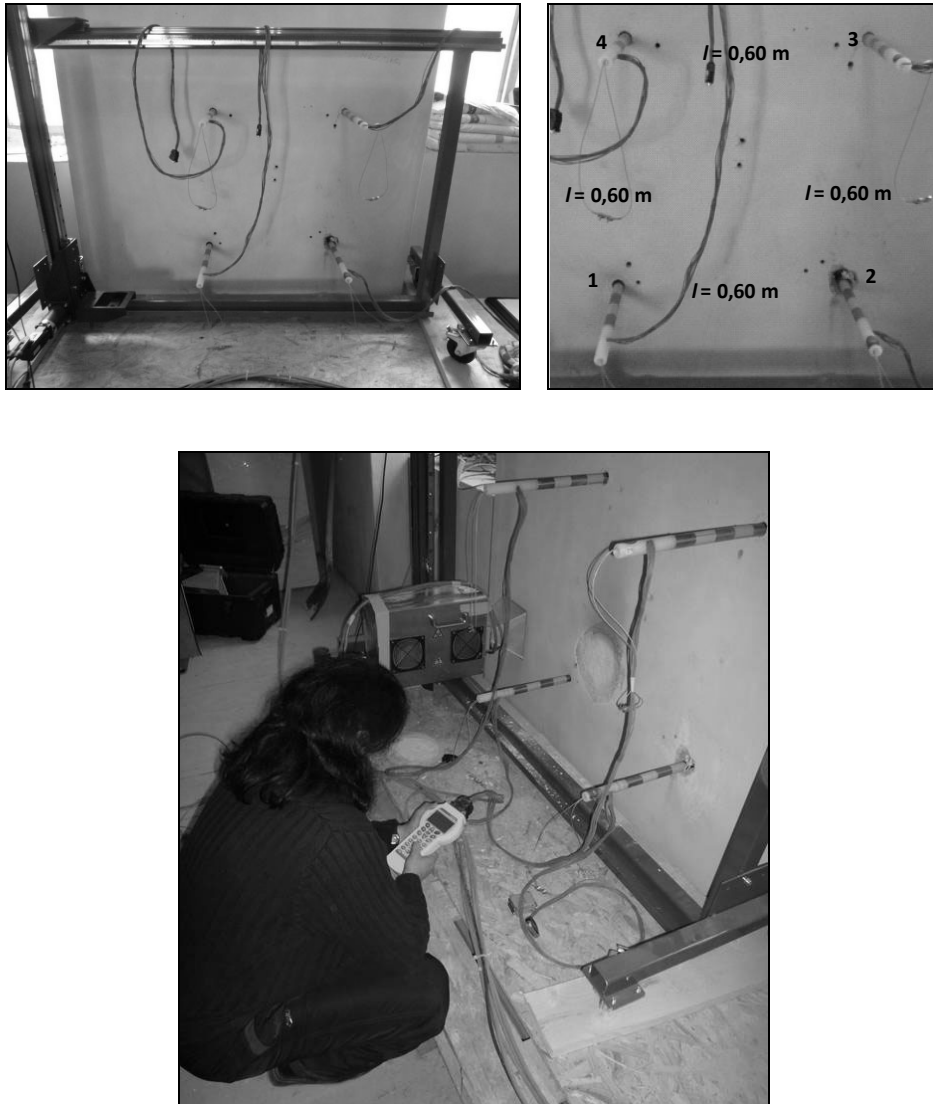
Fig. 17. The impedance measurement (damage to the wall during the application of microwave radiation to a mixed masonry)
