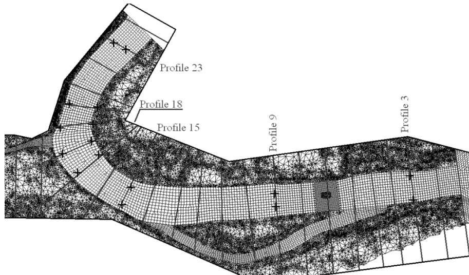
Fig. 3. Position of Profiles and pressure gauging points (crosses)
