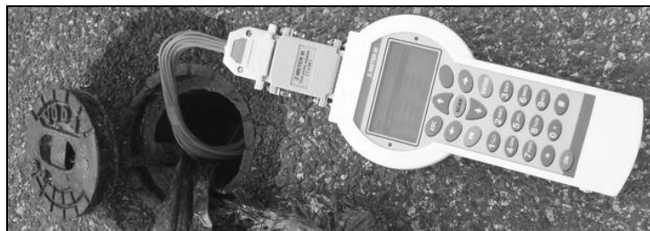
Fig. 3. Structural design of a Z-meter III device with an adapter for measurement on one rod (Karolinka, 2011)
