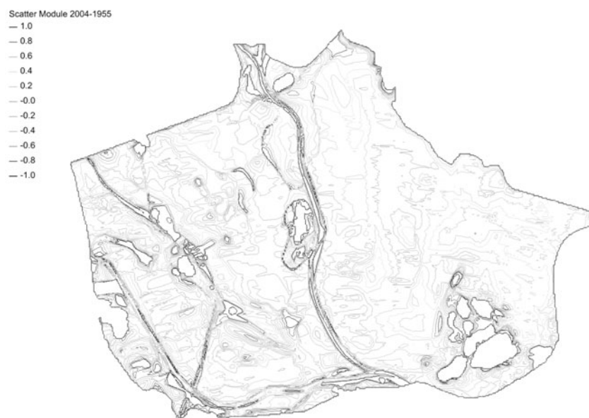
Fig. 2. Differences in the bottom of the middle reservoir – for the years 1981 – 2004
