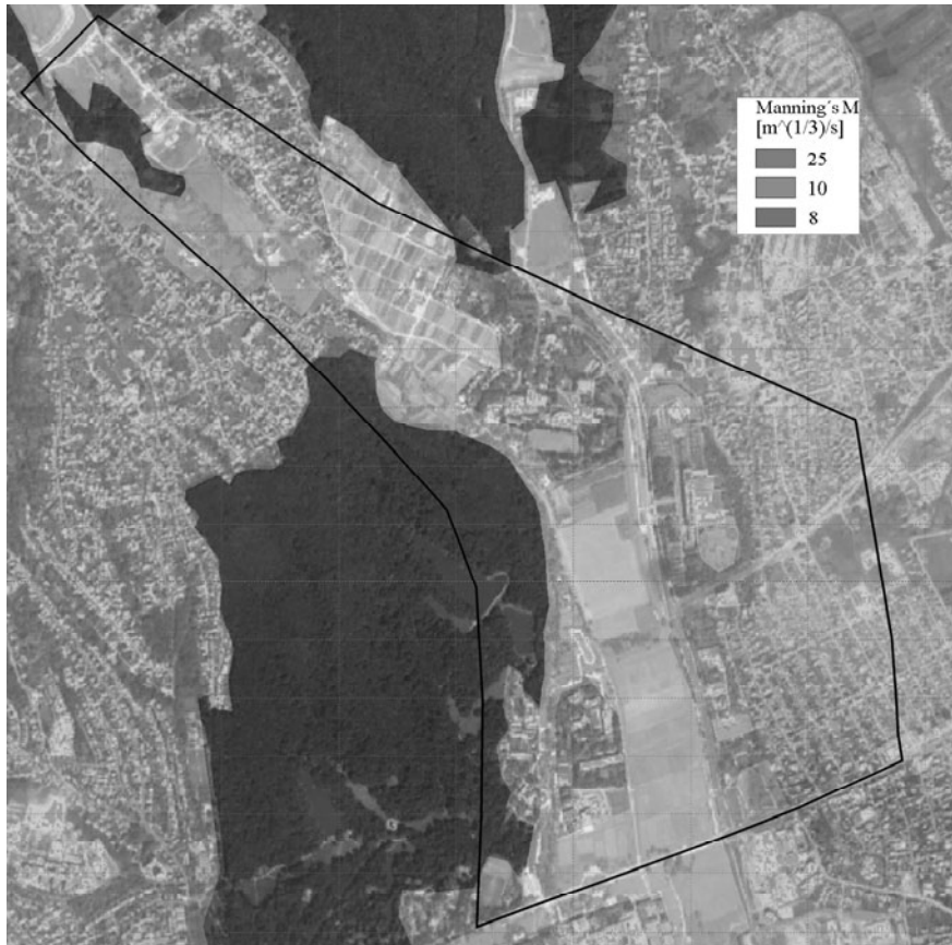
Fig. 3. Modeled area with the adopted roughness coefficient M (Manning's n = 1/M )
