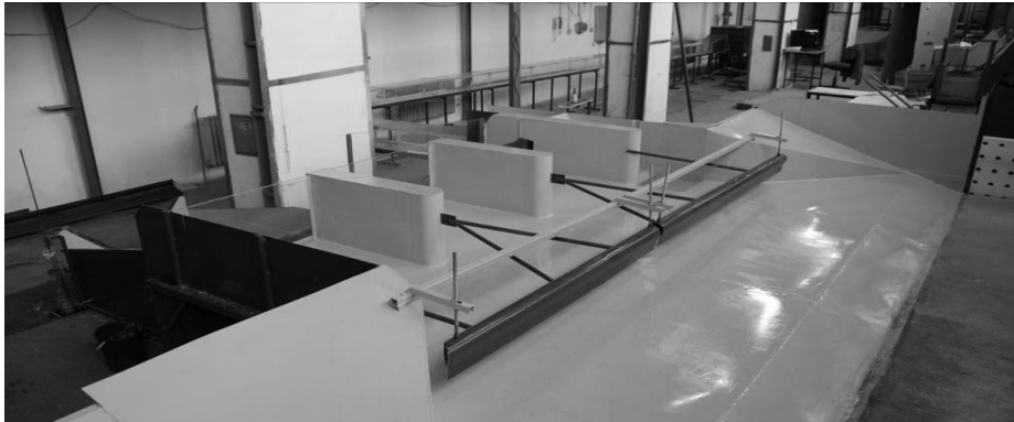
Fig. 3. View on the constructed physical model of the Dobrohošť SHPP in hydraulic laboratory
