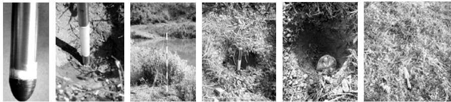
Fig. 3. Composite system of stable measuring electrodes and their installation
