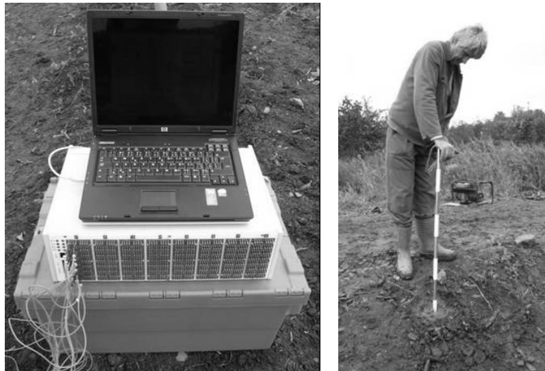
Fig. 1. Z-meter device with control PC and the probes installation
