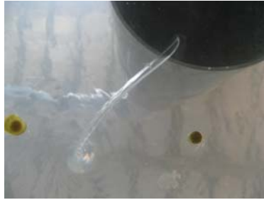
Fig. 3. Vortex formation in the surface of the sump and its connection to suction pipe (Picture is taken from below the sump box)
