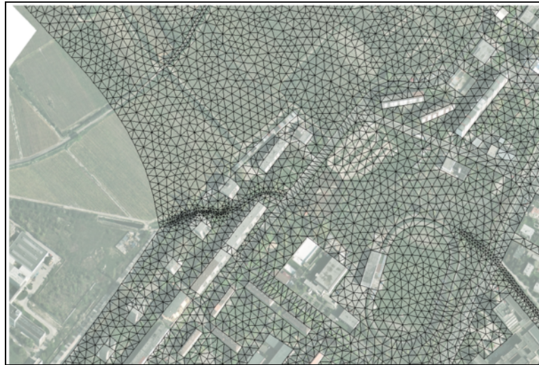
Fig. 7. Detail of the triangular computational mesh
