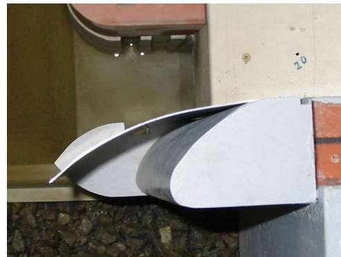
Figure 2 The stream leading plate set on top of the lower part of side pier
