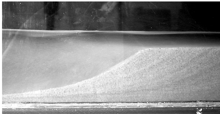
Photograph 2 Movement of sediment through the inflow channel (flow direction from the right to the left)
