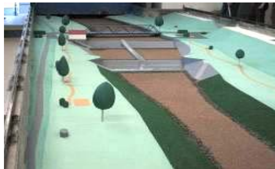
The Hrabovsky weir on Ostravice River with fishway ( M_1 = 50 )
