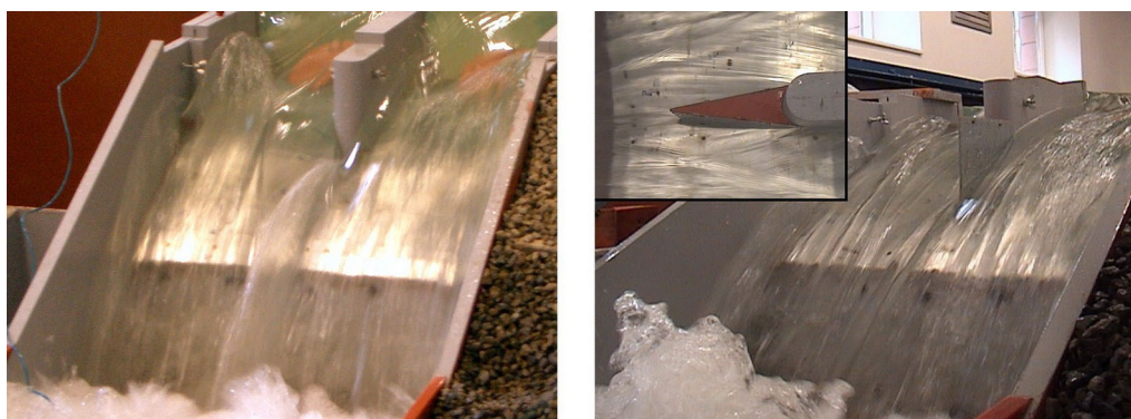
Figure 3 Deformation of level arising behind the end of middle pier and its elimination by the NACA profile when Q = 610 \text{ m}^3 \cdot \text{s}^{-1}
