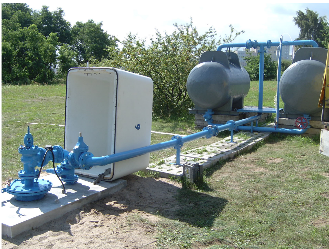
Picture 1 The water meters calibration workstand
