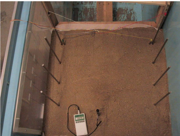
Fig. 6: Four-electrode connection in the monitoring of surface changes
