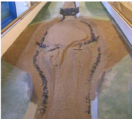
Fig. 4: Watercourse section with the pear-shaped structure – a physical model; a problematic watercourse section due to silting under the weir in Vyšné Lhoty.
