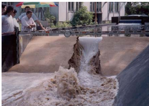
Fig. 4a Breach from the downstream - time 100 s
