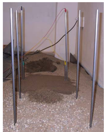
Fig. 6: Four-electrode connection in the monitoring of surface changes
