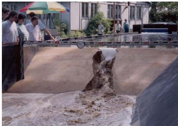
Fig. 3a Breach from the downstream - time 80 s
